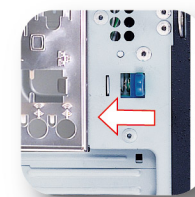
Top cover releasing latch
